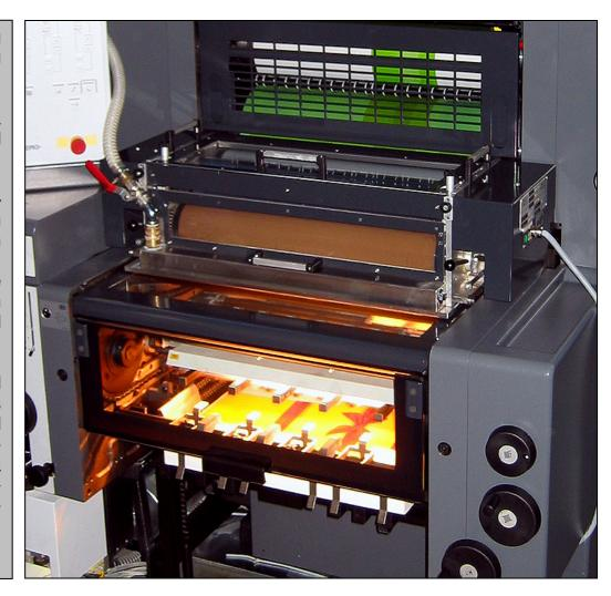
LACO SP 52 coating units are designed as 3- roller systemd, constructed and built of anodised Aluminium and corrosion free stainless steel rollers and parts. Through the electro- mechanical connection to the Plus Version of the press, an absolute synchronized production at all press speeds is guaranteed. The rollers are resistant against UV- coatings, therefore a production with many suitable kinds of water based and UV- coatings as well as with Digital Primers is possible.
